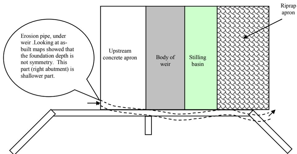
**Figure 3 : The location of seeping pipe under right abutment and concrete body on the plan veiw.**
