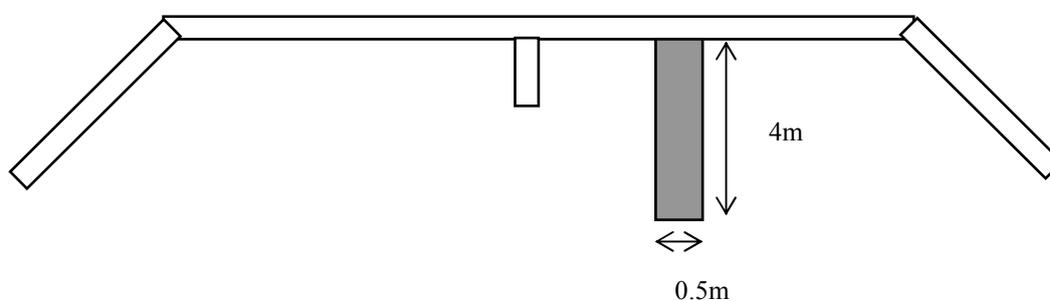
Figure 4: remedial measure for controlling piping at left side of spillway (attached wall is colored section)
